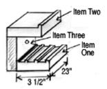
To create the Top Rest, shape the larger piece of wood into an interesting shape (see main photo at top), and then attach the smaller, 1 1/2" wide piece to the underside of it. Then drill a hole through the center of the shaped piece and attach (using a bolt and wing nut) to the top slot on the Center Support.
