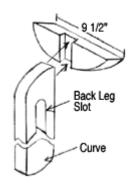
Add the small Front/back connectors as shown in the photos, using small brass screws on the sides of the Center Support (keep them loose so that the Front/back connectors can swing freely) and a bolt through the back leg slot. Note that because the back leg is thinner than the front Center Support, it is necessary to glue an additional scrap of wood onto the back end of each Front/back connector. Having done this, the main frame of the easel is complete.
