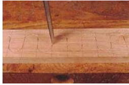
Photo 9- Connect the half circles with a straight bench chisel. Angle these cuts to follow the slope of the design.
