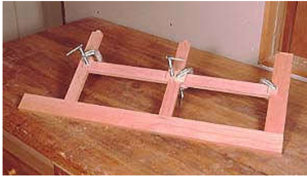
Photo 5- Glue the central dividers (mullions) to the rails before making the panels and gluing up the whole door. Carefully center them on the rails. The long stile is not glued to the rails in this photo, it's just there for alignment. The C-clamps squeeze the mortise walls onto the tenons for a good glue bond. They don't need to be very tight, just light pressure.
