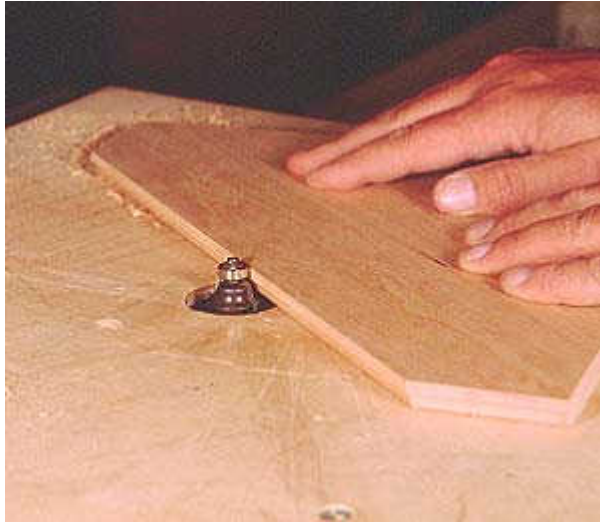
Photo 18- Rout a pattern in to the top edge. Make sure you make the top large enough that the pattern is beyond the top mold pieces.
