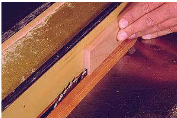
Photo 2- These grooves serve both as mortises for rails and grooves for panels. If your stock is not uniform in thickness, don't flip faces as the text says, because the groove will vary as the thickness does. In this case, always keep the same part face against the fence in all passes and make careful adjustments of the fence location using test pieces to ensure that the groove is as close to centered as possible.
