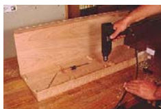
Photo 16- Put the screw blocks in place, and use the holes in them to mark the location of the screws in the carcass. Put a nail in the hole and tap in with a hammer enough to leave a mark. Remove the block and nail, drill for the screw, then install the block. You need to do some tests to determine the optimum hole size and
