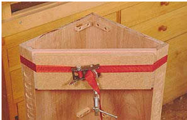
Photo 17- A band clamp (also called strap or web clamp) is the ideal tool for clamping odd shapes like this. The C-clamp just held the spacer in place while the band clamp was installed. An alternative to a band clamp is nylon string. It stretches a bit, so if you wrap it tightly around the piece numerous times the combined wrappings can apply adequate pressure for a good glue bond.
