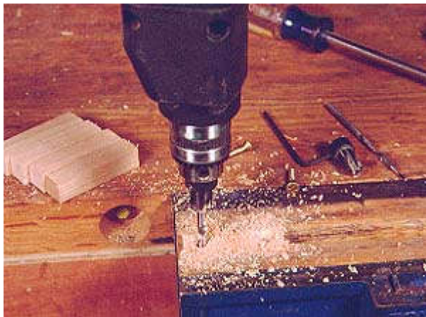
Photo 15- There's a screw block under all those chips from the drill bit! With any screw block it helps to bore out the holes before you go to assembly. This extra step makes the assembly procedure a joy instead of a nightmare.
